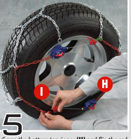
Grasp the bottom tensioner (H) and flip the red lever up to install. Pull the red cable end out and connect to the side chain connector (I). PINCH WARNING: Keep your fingers clear of the chain and tensioner while engaging the tensioners.
