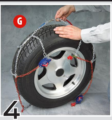
• Leave the red lever in the up position and slide the side cable to the back of the tire (**G**), Ensure the chain is centered on the tire.
