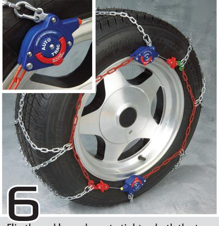
• Flip the red lever down to tighten both the top and bottom tensioners. Your chains will begin to self tighten.
