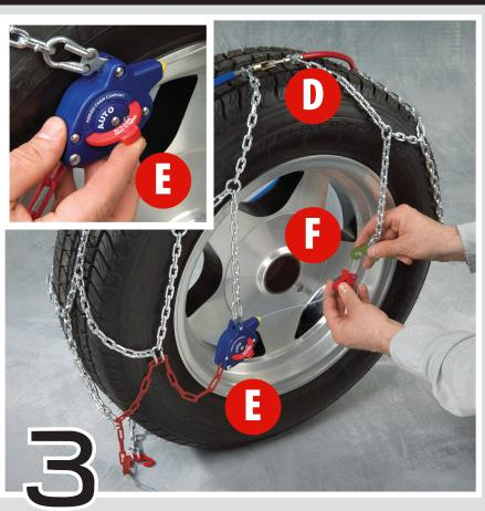
• Grasp the top tensioner **(E)** and flip the red lever up to install. Pull the red cable end out and attach to the green side chain connector **(F)**.
