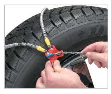
Grasp the outside cable with both hands and pull it toward you to create as much slack as possible. Connect the top fastener (the red one) as tightly as possible by inserting the silver "beads" on the cable through the keyhole.
