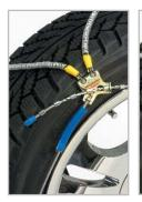
To secure the free ends of the cable, slide the plastic spirals over them with a twisting motion. If insufficient cable
