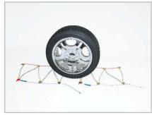
Move the chain is a sweeping motion under the vehicle so the open midsection is positioned up against the backside of the tire. This sweeping motion can best be done while kneeling in front of the tire.
