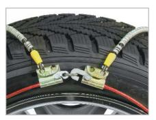
Reach around each side of the tire and grasp both ends of the non-split side cable (that is furthest away from you). Pull both ends to the top of the tire so the fasteners can be seen and manipulated more easily. Connect the inside fastener.
