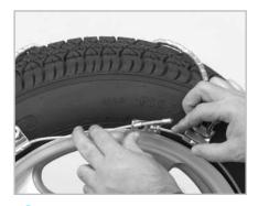
At the top of the outside cable, take the bushing end of the outside split side cable and thread it through the keyhole fastener. Grasp the outside cable with both hands and pull it toward you to create as much slack as possible.
