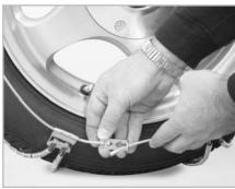
Take the bushing end of the lower fastener and thread it through the keyhole (the one near the ground) using the same process as the top fastener. Please see below for a detailed look at making this connection.
