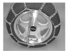
Attach the rubber tensioner to take up the additional slack. To make this simpler, attach the first hook at the "5 o'clock" postion and the second at the "11 o'clock" position and so forth. Tighteners must be purchased separately,
