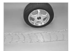
Park vehicle on firm level ground and turn off the engine. Set the parking brake. Unroll the chains and lay them out flat making sure there are no twists or tangles. Make sure the smooth side of the cross chain hooks are toward the tire.
