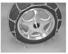
Drape the chain over the tire, again making sure cross chain hooks are facing upward. Hooks that face down (towards the tire) will cause damage to the tire.
