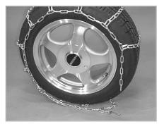
Pull one cross chain down to the point where the tire meets the ground. Move the vehicle so that 1 or 2 cross chains pass under the tire.
