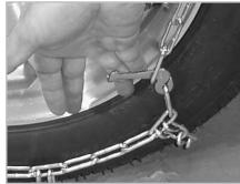
5 Next fasten the outside fastener, making sure it is as tight as possible. Drive a short distance and retighten all fasteners. For best results, make sure fasteners are adjusted equally and as tight as possible.
